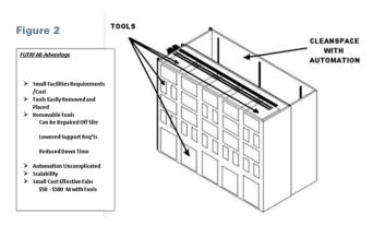
Vertical Tools: Tools densely packed in arrays can be removed, repaired, and replaced without entering the fabrication space. Distance between tools is also much shorter, making automation simpler and more efficient. Even the tools themselves can be small enough to operate efficiently at a 2-inch wafer size (as opposed to today's 12-inch wafer.)
